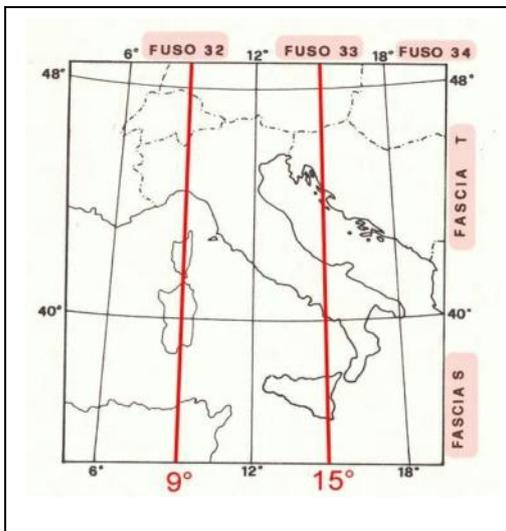
Figure 3. UTM zones for Italy. In red the central meridian of the zone.
