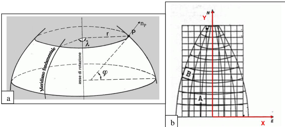
Figure 1. a) geographic reference system ( $\lambda$  = longitude,  $\phi$  = latitude); b) planimetric (or cartographic) reference system
