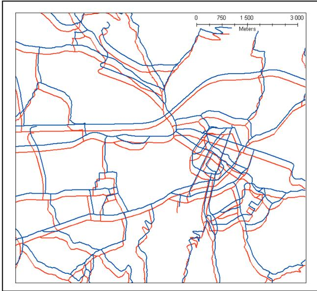
Figure 2. Effects of datum offset. The blue road network is correctly assigned with the WGS84 datum; the red network is the same as the blue one, but a wrong datum (ED50) was assigned to it. The projection is UTM33 for both.
