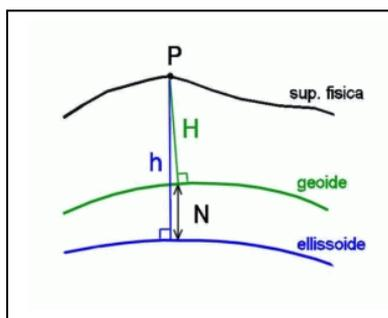
Figure 4. Geodetic (h) vs. topographic (H) elevation.
