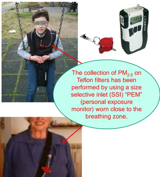
Figure 1. Volunteers wore a SKC sampler (flow rate 10L/min) equipped with a PM<sub>2.5</sub> particulate selector
