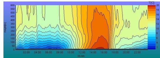
Figure 6. MTP-5P microwave radiometer temperature profile collected at Tor Vergata.
